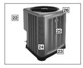
The Variable Speed compressors (28) with standard internal pressure relief and internal thermal overload are used on all capacities assuring longevity of high efficient and quiet operation for the life of the product. All RP20 Heat Pump come standard with high and low pressure transducers reinforced vinyl compressor sound covers containing a 11/2 inch thick batt of fiberglass insulation and open edges are sealed with a 1 inch wide hook and loop fastening tape for superior sound quality.
